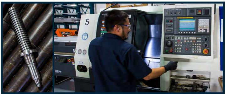
Top Left - This acme shaft was the reason Garner added CNC turning. Top Right - The Hyundai Wia CNC 150A with bar feeder runs only 6 part numbers, but each one of them is critical to the trouble free operation of their products. Right & Right Middle- Garner Products has three YCM NXV 1020A mills and two Fadals. The Fadal 3020 has a 4th axis. Bottom Right - A sampling of internally produced parts shows the variety of shapes and materials used in their data destruction devices.
